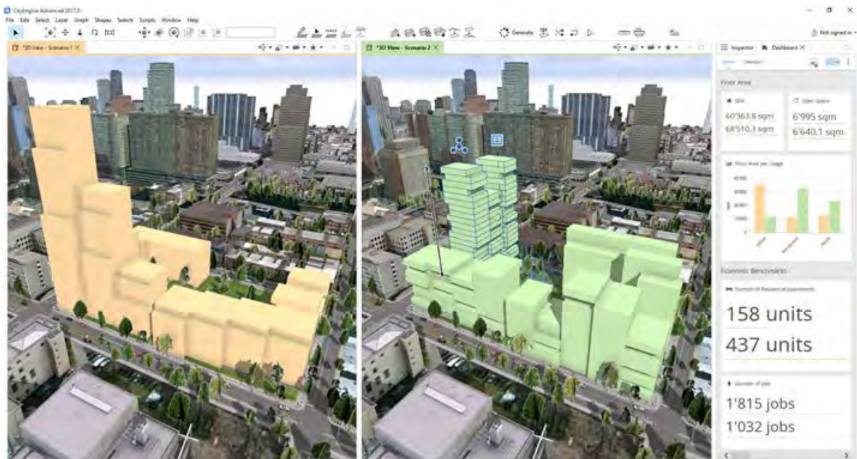
Fig.3: Typical side-by-side presentation of alternative massings for a new urban development (Source: Esri)
