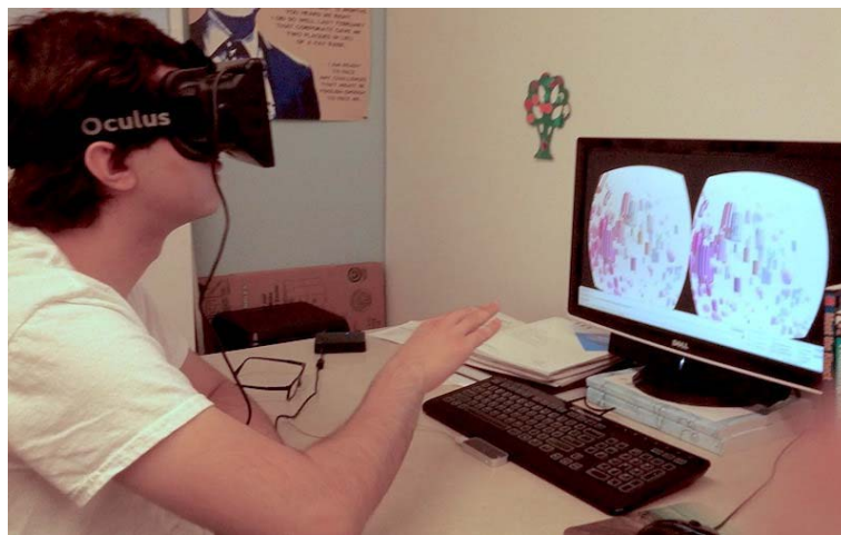
Figure 2.1: iViz. A student navigating through the visualized data space, using the Oculus Rift VR headset and Leap Motion gesture control (Donalek et al, 2014).
