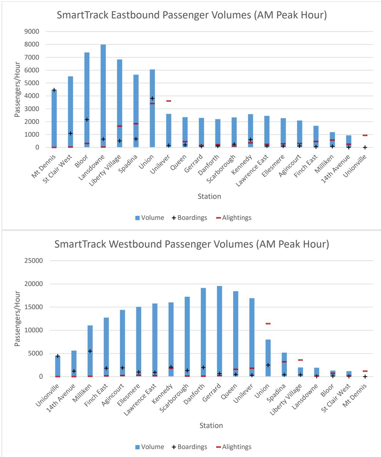
**Figure 4.10: 2031 AM Peak Hour SmartTrack Loading by Line Segment\***
