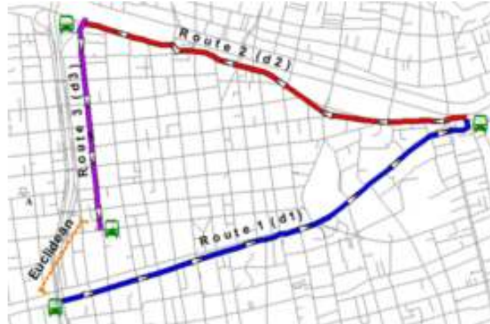
Figure 2. A three-legged trip comparison between Euclidean and on-route distance (from Munizaga et al., 2014)
